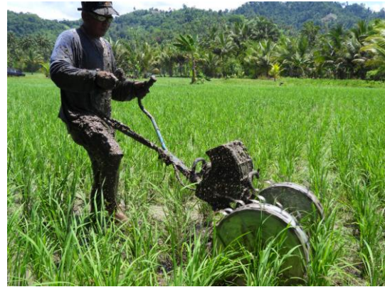
Rotary power weeder from AfricaRice.
