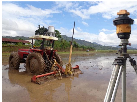
Laser-guided land leveling system with tractor.
