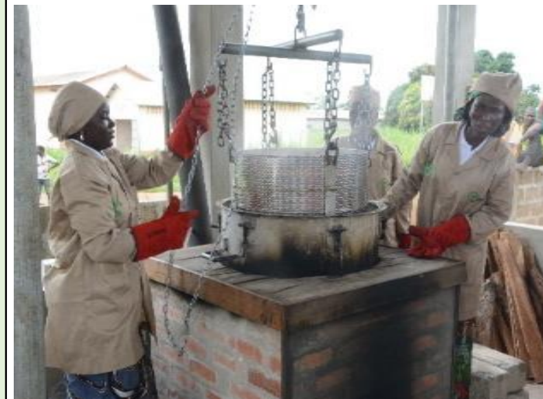
Parboiling Rice by RINA SARL Enterprise in Cote d'Ivoire – conditioning paddy for milling
