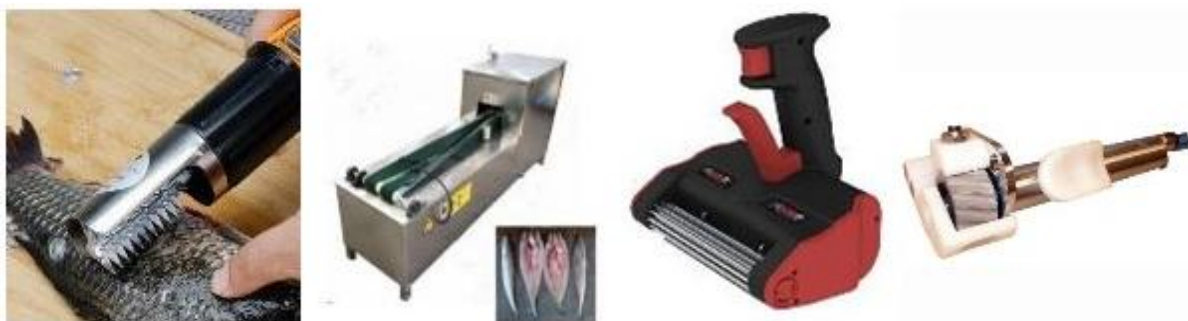
Range of fish processing tools (left to right): scaler, cutter, Skinner, and de-boner
