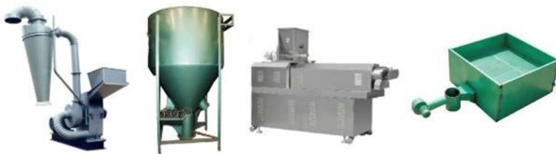
Fish feed production line (left to right): hammer mill, vertical mixer, extruder, and dryer
