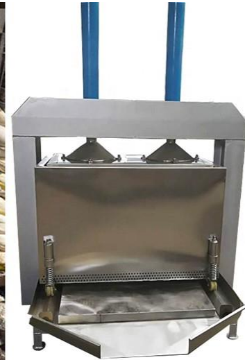
A fabricated gari screw press in operation (left) and a hydraulic press suitable for commercial production (right)
