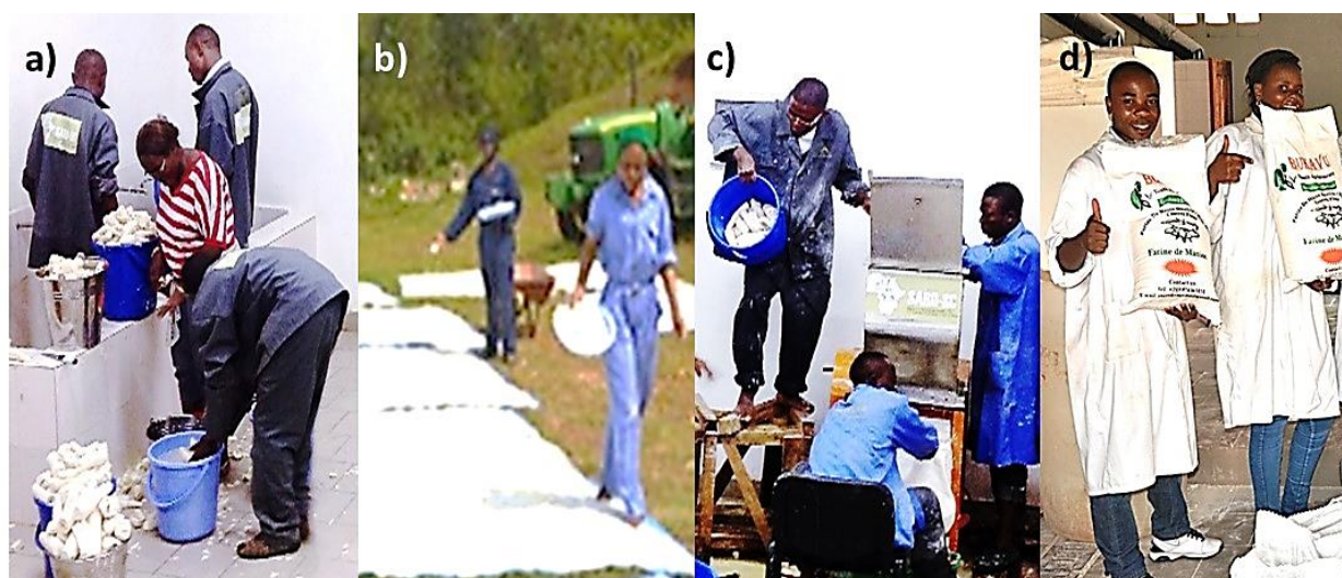
A “low-tech” youth-led cassava flour factory in action: a) washing and shredding peeled cassava roots, b) air drying shredded roots, c) milling dried roots into flour, d) displaying the finished product
