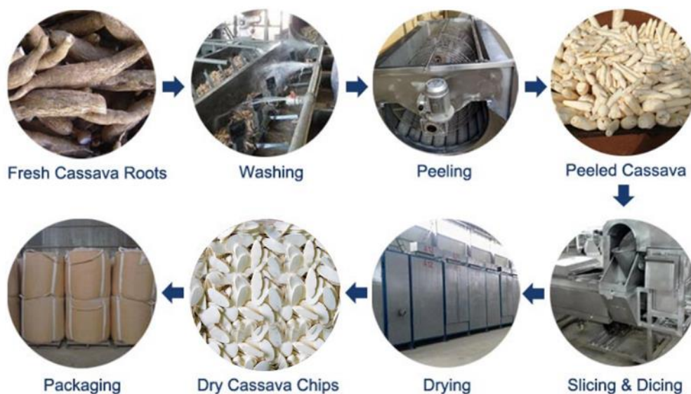
Steps of large-scale cassava chip production process.
