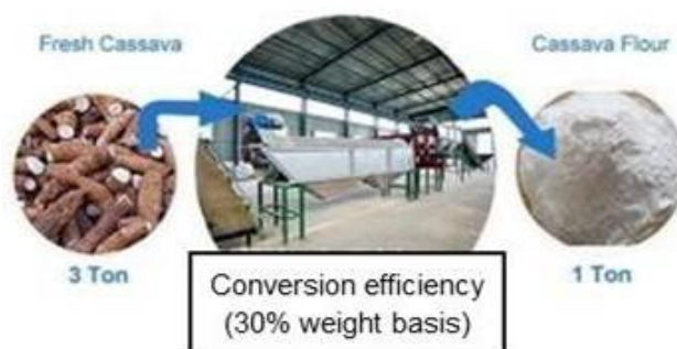
The conversion of fresh cassava root to high quality cassava flour
