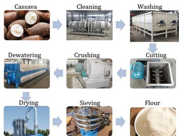
A modern industrial cassava flour processing approach where all operations are mechanized (from: cassavaprocessing.com)
