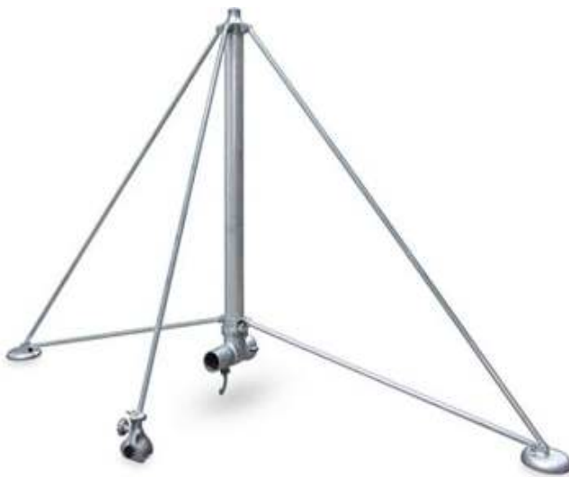
The stand of a rain gun; note that water enters from the base through a threaded fitting and is delivered to the rain gun mounted at its top
