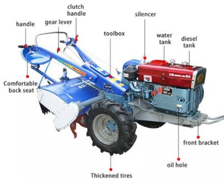
A top of the line two wheel tractor available in China, note that it includes a seat for the operator
