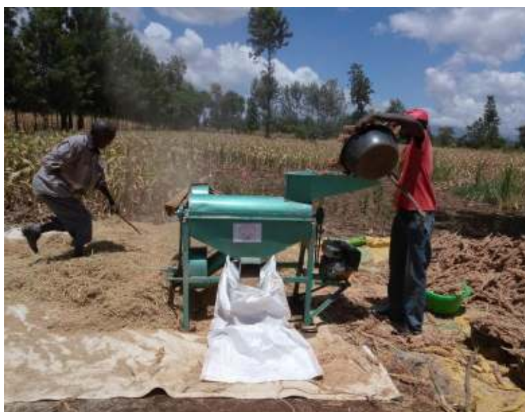
Power thresher processing sorghum grain
