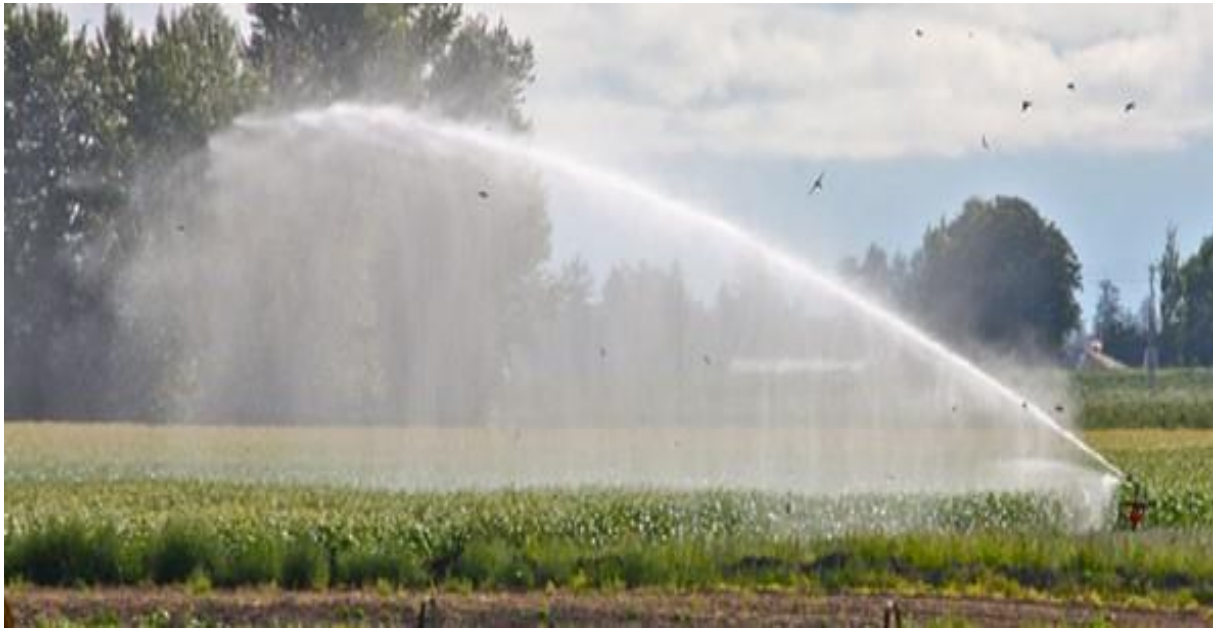
A high-pressure, high-volume rain gun in operation, projecting irrigation water up to 60 m from a single field position
