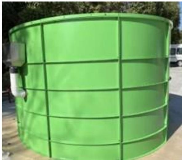
*A batch digester for producing biogas from poultry manure*
