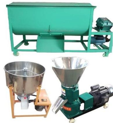
*A horizontal mixer (top), mill (left) and pellet machine (right) used in small-scale feed production*
